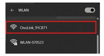
After connecting to the Onolink access point (**onoLink\_XXX**) and opening the configuration page (**192.168.4.1**), the configuration screen will appear as shown below:
